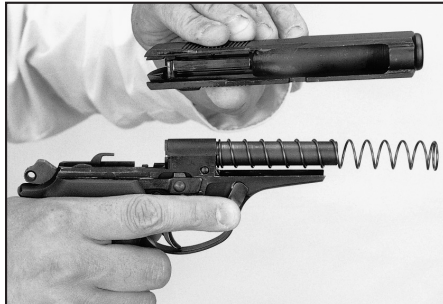
Disassembly of the Series 95 begins with removing the magazine and making sure the chamber is empty. Press down on the disassembly lever at the frame's right, then pull back and up on the slide, allowing it to move forward and off of the gun's frame Walther-style.
